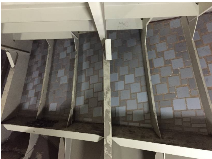
Soundac® PU-D30 applied on a ship hull
